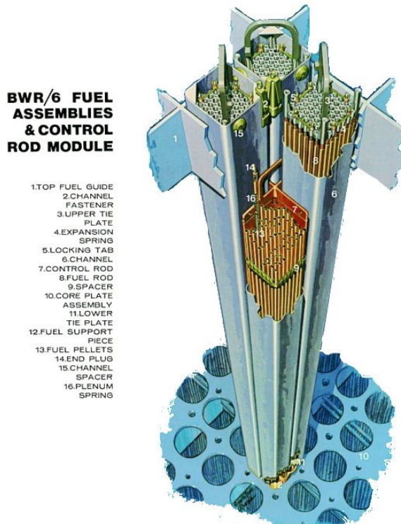
Fig. 2. Sketch of a single fuel bar in a solid-core, commercial Boiling Water NR
